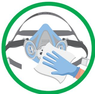
Disinfect by soaking, wiping, or spraying the facepiece according to facility protocol and User Instructions. Rinse thoroughly with fresh warm water. Air dry in a non-contaminated area.
