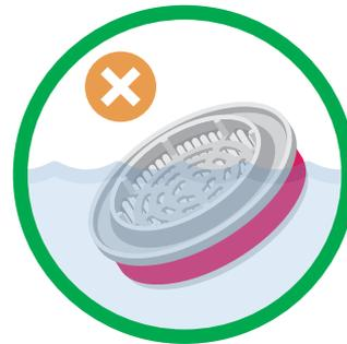
Filter cartridges must not be dipped or immersed in a cleaning or disinfection solution because this may damage or render the filter material ineffective. When using a cleaning or disinfectant wipe on the external surface of a filter cartridge, users should avoid contact with the filter media on the inside of the cartridge.
